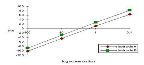
Graphing the electrode potential (in mV) versus the log of concentration (mg/L) gives visual feedback that the electrode response is fairly linear over this concentration range.
