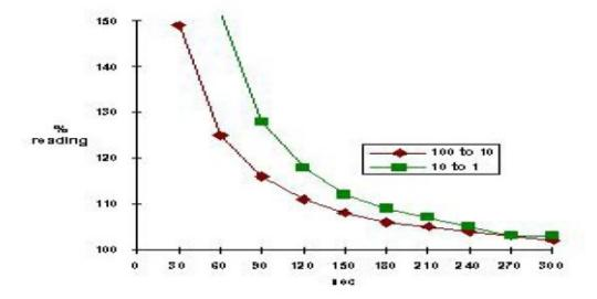
As the above response time graphs show, upon going from lower to higher concentration the electrode provides a stable signal in about 2 to 3 minutes, with slower response at the lower end of the working range. Upon going from higher to lower concentrations, however, the gas-sensing probe requires considerably more time, on the order of 5 or 6 minutes to reach a stable signal.
